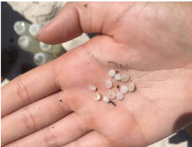
Figure 3. Nurdles, a form of primary microplastics, found on a beach in Mississippi. (Photo by Mandy Sartain)
