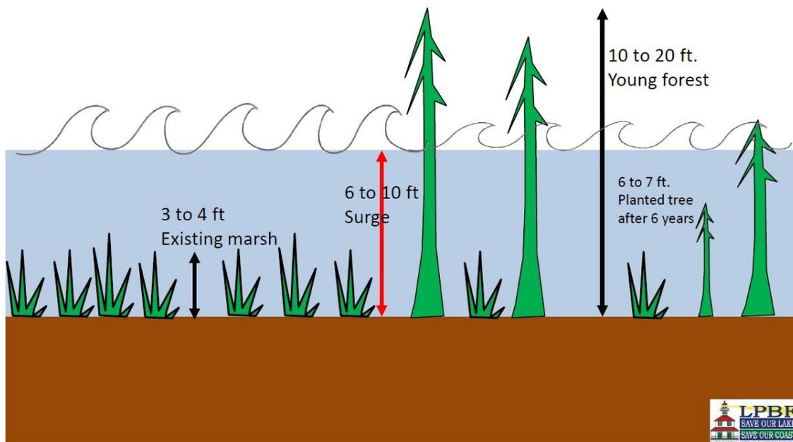
**Fig. 1: Schematic diagram of storm surge and wave action on a marsh versus swamp. The diagram is meant to illustrate the greater dampening effect forest trees have on surge as opposed to marsh.**
