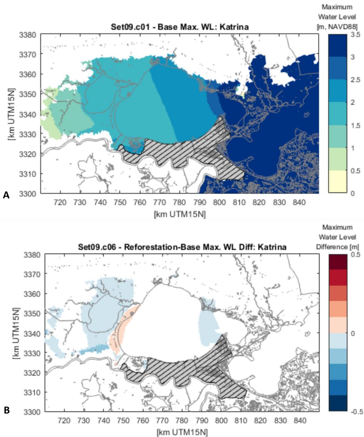
**Fig. 3: A) Maximum water level from Hurricane Katrina using the present landscape. B) Difference in water level between the base case (water level in A) and the maximum water level with a reforested Maurepas land bridge.**
