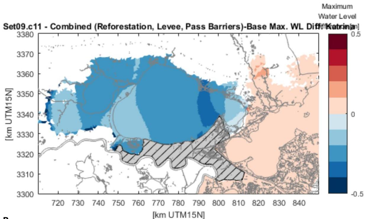
**B** Fig. 4: A) Difference in water level between the base case and the maximum water level with a reforested Maurepas land bridge, West Shore Lake Pontchartrain levee, and barriers on the Passes for Hurricane Isaac. B) Difference in water level between the base case and the maximum water level with a reforested Maurepas land bridge, West Shore Lake Pontchartrain levee, and barriers on the Passes for Hurricane Katrina
