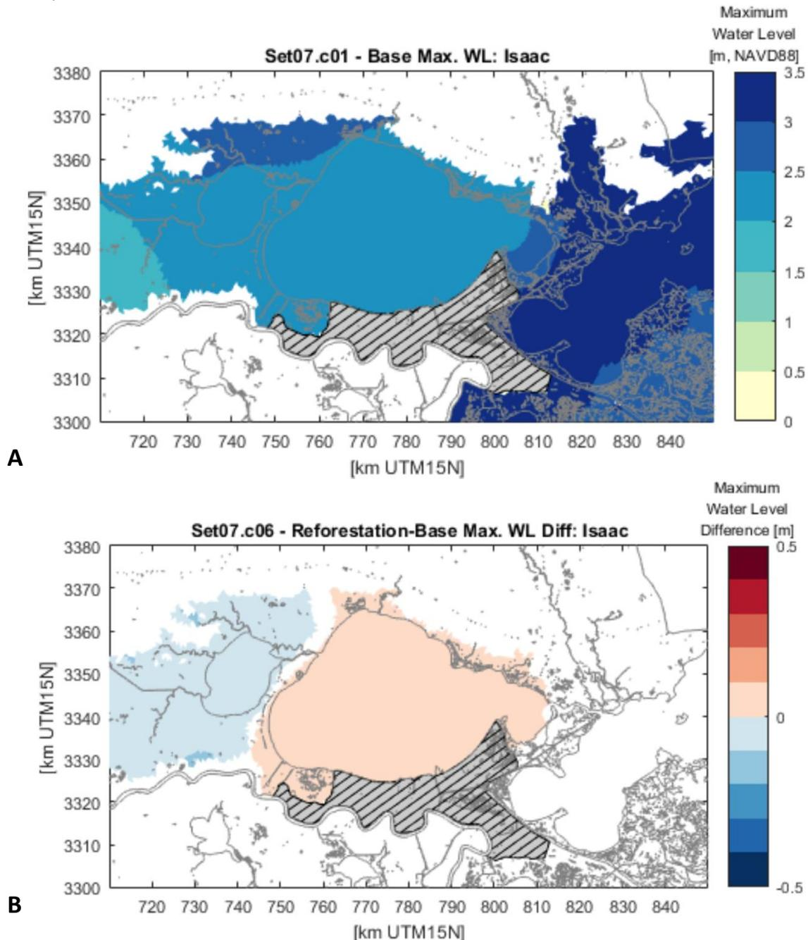
**Fig. 2:** A) Maximum water level from Hurricane Isaac using the present landscape. B) Difference in water level between the base case (water level in A) and the maximum water level with a reforested Maurepas land bridge.
