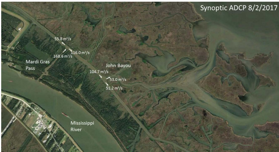
Figure 4. Mardi Gras Pass flow and flow distribution in the receiving basin at key junctions in the back levee canal and John Bayou.
