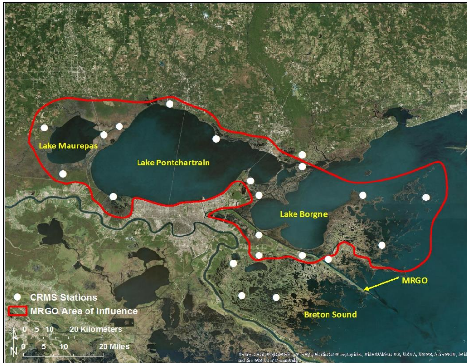
Figure 4: Estimated influence area of the Mississippi River Gulf Outlet (MRGO) in the Pontchartrain Basin. Using the soil salinity data at the Coastwide Reference Monitoring System (CRMS) stations, the area of influence was predicted to be 525,207 hectares (over 1.2 million acres).
